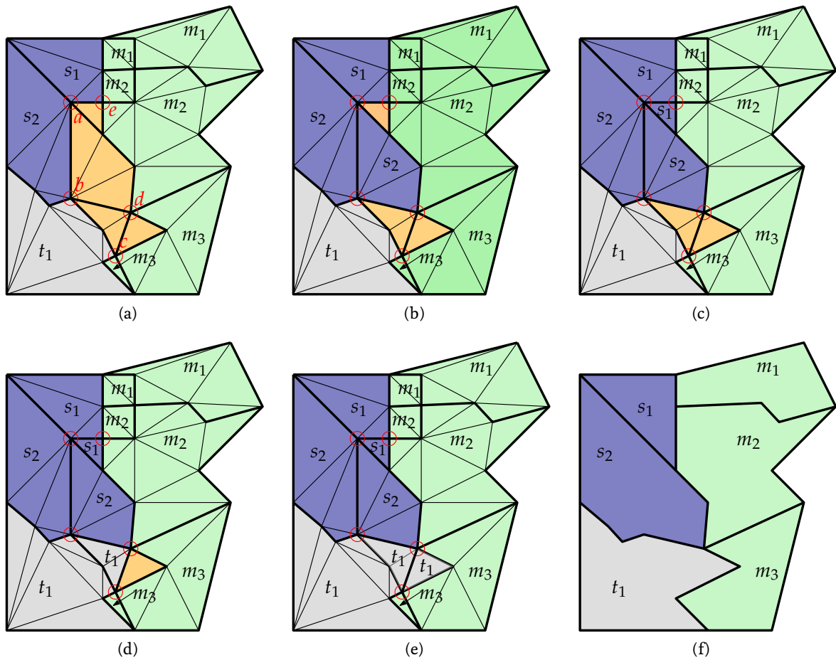
Figure 8: The same three input datasets as in Figure 7. The overlapping regions have already been repaired. (a) 5 split vertices are identified ( a, b, c, d , and e ), and 3 extra constrained edges are inserted in the CDT ( bd, cd and the one incident to a ), separating the gap region into 4 sub-regions. (b) The sub-region adjacent to s_2 is relabelled. (c) The sub-region adjacent to s_1 is relabelled. (d) The sub-region adjacent to t_1 is relabelled. (e) The last sub-region is relabelled (to t_1 ). (f) The resulting aligned datasets.
