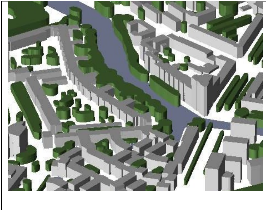
Figure 21: LOD1 of a Vegetated Terrain Area, together with a LOD1 building (source: iDelft)
