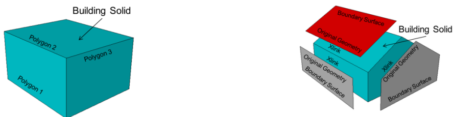
Figure 10: Left: An LOD1 solid (without surfaces) Right: An LOD2 solid with accompanying modelled surfaces (image taken from CityGML specifications)
